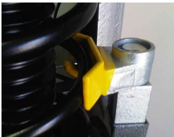
Correct hook engagement on spring coil.
