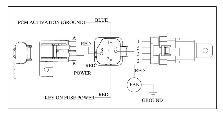
NOTE: If the fan connector on the relay kit does not work with your fan, you can replace your fan connector with the one provided in your PSI Fan relay kit.
