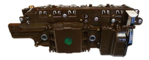
Note: TCM held in place with external torx-plus bolts (not a standard socket configuration).
